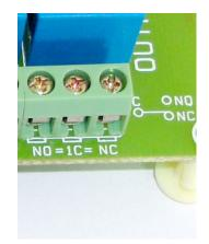
For example, When you want to switch on light when relay comes on, then the light has to be powered through C and NO contacts. In this case NC will not be used.
