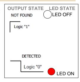
The output is active low and can be given directly to microcontroller for interfacing applications.
