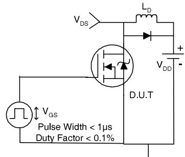
Fig 16. Switching Time Test Circuit
