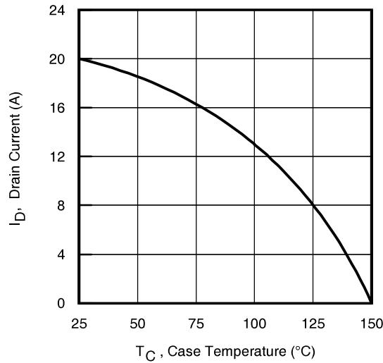
**Fig 9.** Maximum Drain Current Vs.
