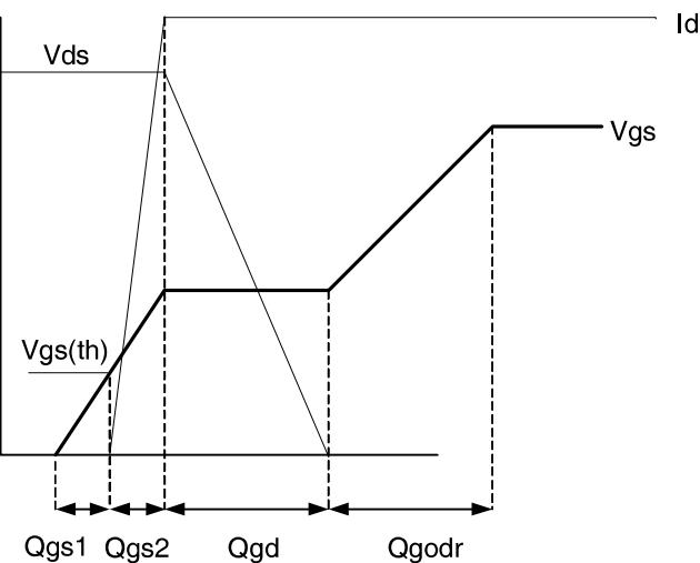
**Fig 19. Gate Charge Waveform**
