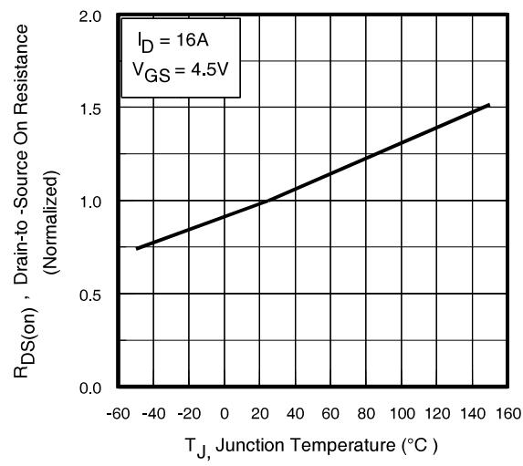
**Fig 4.** Normalized On-Resistance
