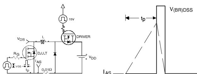
Fig 14. Unclamped Inductive Test Circuit and Waveform
