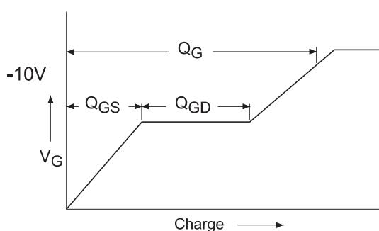
**Fig 13a.** Basic Gate Charge Waveform
