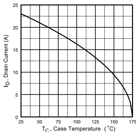
**Fig 9.** Maximum Drain Current Vs.
