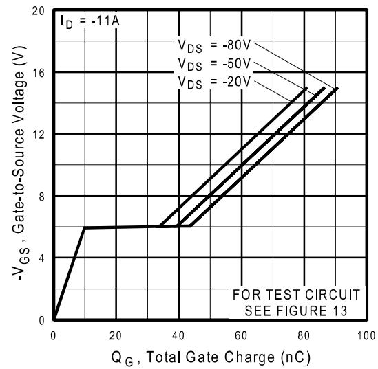
**Fig 6.** Typical Gate Charge Vs.
