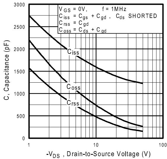
**Fig 5.** Typical Capacitance Vs.
