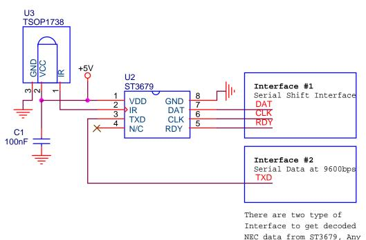
Two types of Interface for reading NEC data from ST3679
