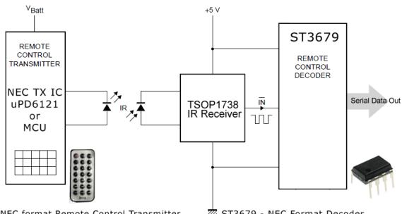
NEC format Remote Control Transmitter http://www.sunrom.com/p-1022.html ST3679 - NEC Format Decoder http://www.sunrom.com/p-1044.html
